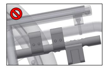
Now mount the complete adapter bar that consists of center pipe (A), outer pipe (B) and clamp (C). The complete adapter bar is mounted into the holders (D) by using the QR-pins (E).
