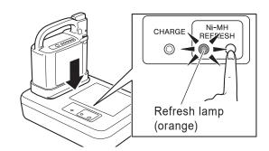
(2) The refresh lamp (orange) changes from a flashing to an "on" state, and the refresh charging starts.
