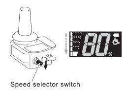
(3) After releasing the switch once, hold the speed selector switch down and you will hear the beep sound.
