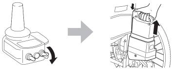
② Switch the left and right clutches to the power drive position.
