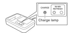
While in standby mode, when the battery reaches an appropriate temperature, the charge lamp (green) will change from a flashing to an "on" state, and charging will start automatically. (The length of the standby time varies with the conditions.)
