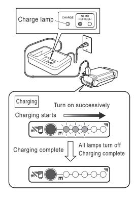
After charging has completed, unplug the charger plug and the power plug, then securely close the battery's connector cover.
