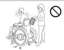
While the wheelchair is being operated or after operation, do not touch the back of the drive units. During or after operation, the back of the drive units may be hot. In addition, if the wheelchair is near a source of heat, the drive units may become hot.
