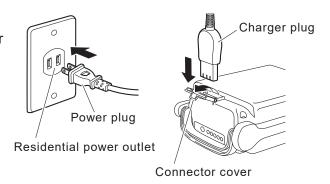
TIP After plugging in the charger, it takes about 5 seconds for the charging lamp to light.
