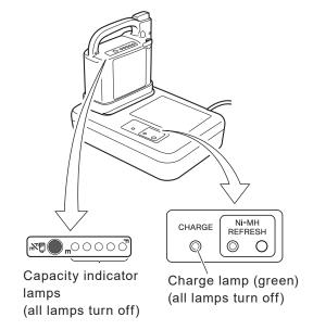
After charging is complete, you can check the charged capacity by pressing the battery indicator switch.
