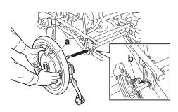
Push in each power unit completely. Check to ensure that the two balls "a" on the end of the axle can be seen completely.
