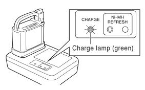
• The battery temperature increases during charging. However, if the battery temperature rises above 50°C, the power for the charger will turn off to protect the battery.
