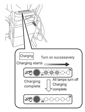
② After charging has completed, unplug the charger plug and the power plug, then securely close the battery's connector cover.
