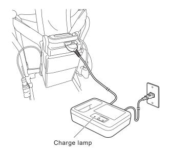
While charging, you can check the charge status using the capacity indicator lamps on the battery.
