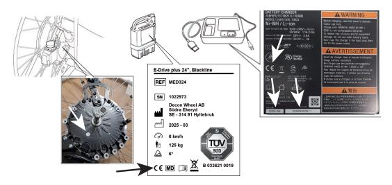
CE marks are placed on the motor, on the battery, and on the battery charger, which even is marked with registration number including the production year and month.
