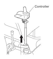
(4) Insert the controller into the lower holder.
