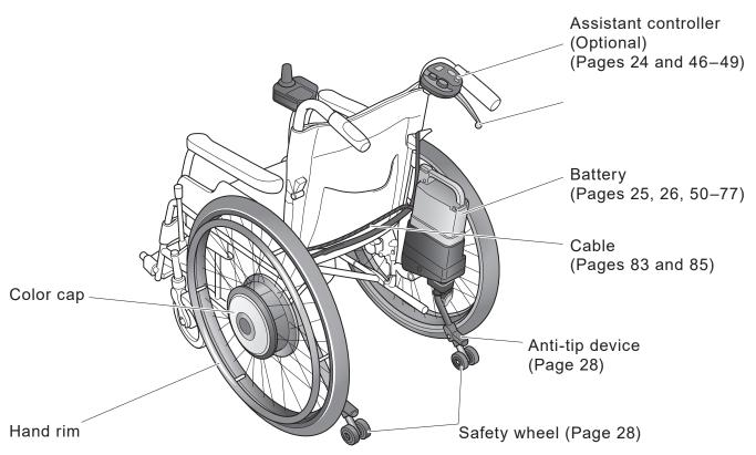
Either a nickel hydride battery set or a lithium ion battery set is supplied.
