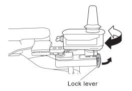
(3) After release the lock lever, the controller position is fixed with lock position.
