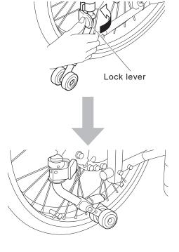
(2) Returning the retracted anti-tip device to its original position
