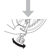
Make sure that the anti-lock device is locked in position.
