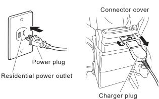
© Check that the charge lamp (green) on the charger turns on.
