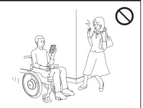
Do not operate the wheelchair near a device that produces strong radio waves. If the wheelchair is near a source of radio waves and starts to operate abnormally, immediately turn off the power, and quickly move away from that location using the assistant operations or manual operation.
