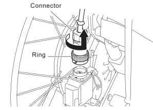
On models that feature an integrated battery seat, the connector is located on the left wheel.
