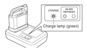
If the charge lamp (green) does not turn on, and the refresh lamp (orange) flashes, refer to "8.5. Refresh Charging the Nickel Metal Hydride Battery (JWB2)".
