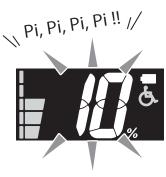
(3) Once the battery runs out, the residual capacity indication changes to "E" and flashes, a long buzzer beeps "Pi—" once and stops.
