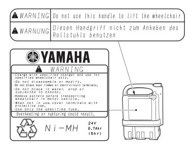
Ni-MH and Li-ion combined Charger (ESC3)
