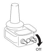
(2) Turn the controller while the lock lever of the holder is pushed forward.
