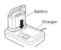
TIP After plugging in the charger, it takes about 5 seconds for the charging lamp to light.
