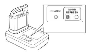
In a refresh charging process, after all remaining electricity has been discharged, the refresh lamp (orange) turns off. The charge lamp (green) comes on and a normal charging process begins. The time it takes from the start of refresh charging to the completion of normal charging is 3-19 hours.
