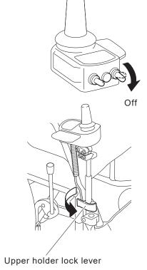
(3) Pull the controller upward to remove it.
