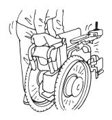
(8) Secure the wheelchair. Secure the wheelchair to prevent it from moving or hitting any surrounding objects.
