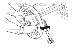
Place the power units in their normal position, and then apply the parking brakes.
