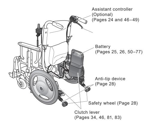
Either a nickel hydride battery set or a lithium ion battery set is supplied.
