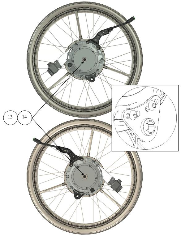
3. Check the correct placement for the eMove, and that it is axle Ø12,0 x 51 with Part Number: XOE-2530-BO and Spacer with Part Number: XOE-25383-00.
