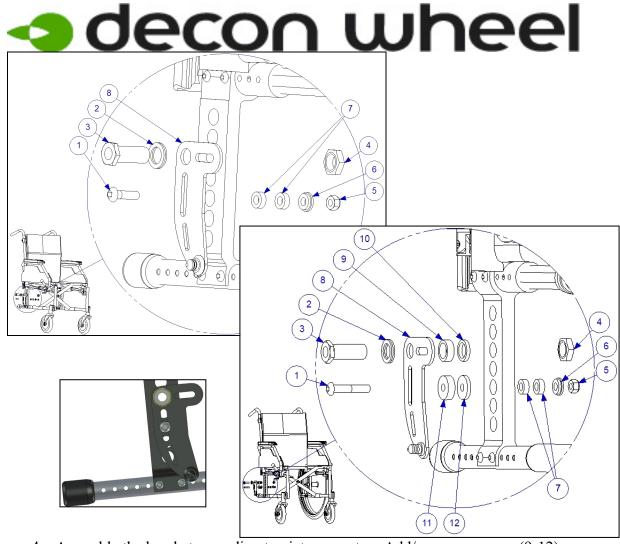
4. Assemble the bracket according to pictures on top. Add/remove spacers (9-12) depending of what type of adapter plate and what placement it is.
