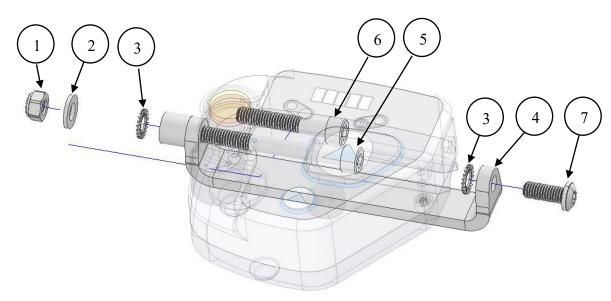
Use either a bolt with position 4 or 5 depending on which clamp is mounted on the chair's handle tube. The shorter one fits the sheet metal clip and the threaded aluminum clip, the longer aluminum clip without threads.
