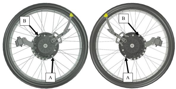
2. Make sure that the stop pin without washer is in accordance with the pictures above, and that the anti-tip guard is removed.
