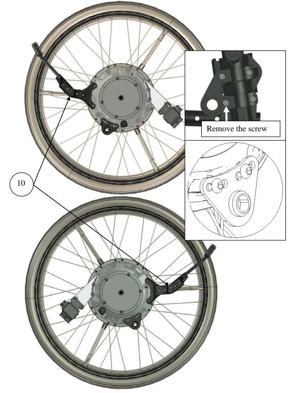
2. Check the correct placement for the eMove with axle Ø12,7 x 46 with Part number: XOE-2530E-00
