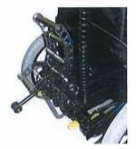
**Illustration 17: Connecting and** disconnecting the drive function
