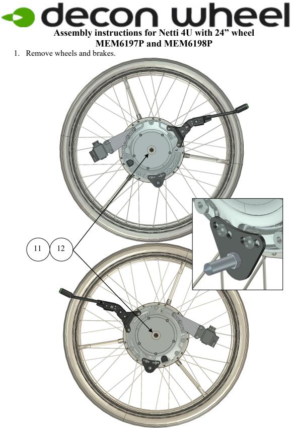
2. Check the correct placement for the eMove, and that it is axle Ø12,0 x 51 with Part Number: XOE-2530E-BO and Spacer with Part Number: XOE-25383-00 and Stop pins are assembled with Part Numbers: 290000, 300001 and XSM8ML.
