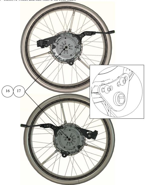
2. Check the correct placement for the eMove with axle Ø12,7 x 51 with Part number: XOE-2530E-C0 and Spacers with Part number: XOC-25383-00
