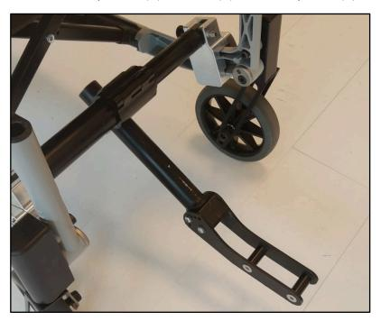
Mount the adjustment toll onto the fork (B). Remove the screws in the fork that locks the rotation (see picture bellow). Also make sure that the fork sits in the center of the wheelchair.
