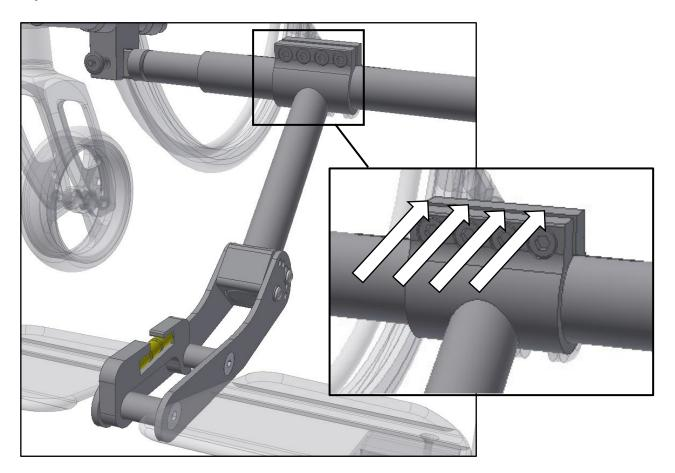
Check one last time that all screws are properly secured. Now see the user manual of Adventus to continue the installation. This can be downloaded from <a href="https://www.decon.se/en/">www.decon.se/en/</a>
