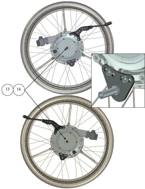
2. Check the correct placement for the eMove with axle Ø12,0 x 51 with Part number: XOE-2530E-B0 and Spacers with Part number: XOE-25383-00 and Stop pins are assembled with Part Numbers: 290000, 300001 and XSM8ML.
