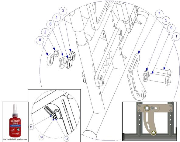
3. Assembly of the plate (right side) and the brake extender according to pictures. Parts for right side mounting:
