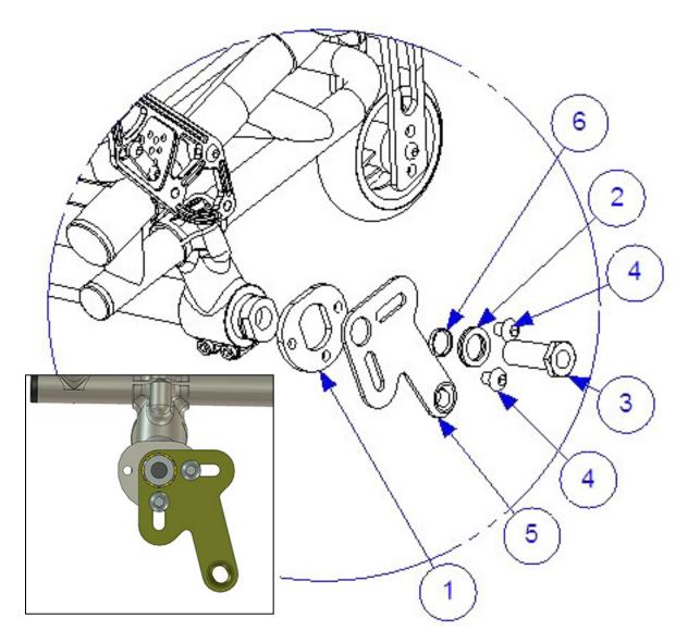
3. Assembly the plate (right side) according to picture. Parts pair mounting set for right side:
