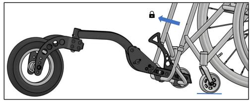
Swing the wheel backwards so that the castors are lifted off the ground.
