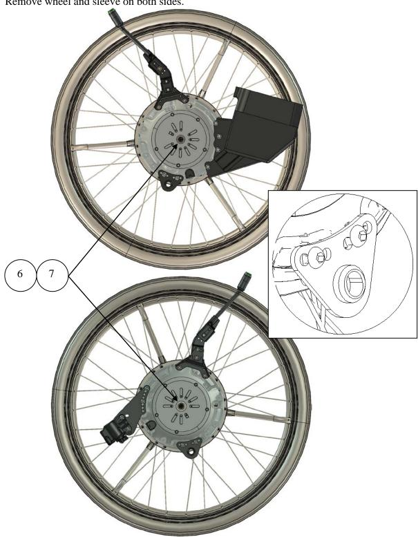
2. Check the correct placement for the eMove, and that it is axle Ø12,7 x 55,5 with Part Number: XOE-2530E-AO and Spacer with Part Number: XOC-25383-00.
